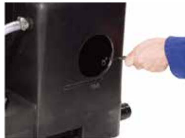
清理毛刺 Deburring inlet hole
