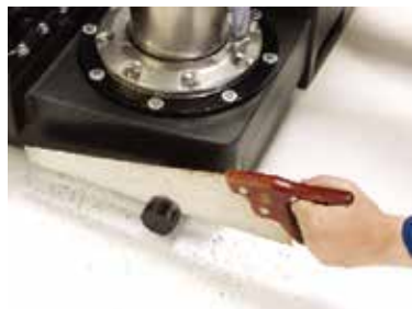
给手动隔膜泵开接口 Open up suction connection to diaphragm hand pump
